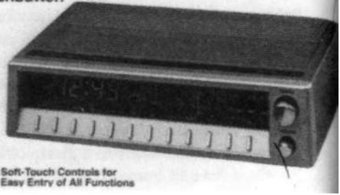
**4.5 A Clock Radio, "Human Engineered" to Simplify Operation.** Note the row of identical-looking switches. (Copyright Tandy Corporation. Used with permission.)
