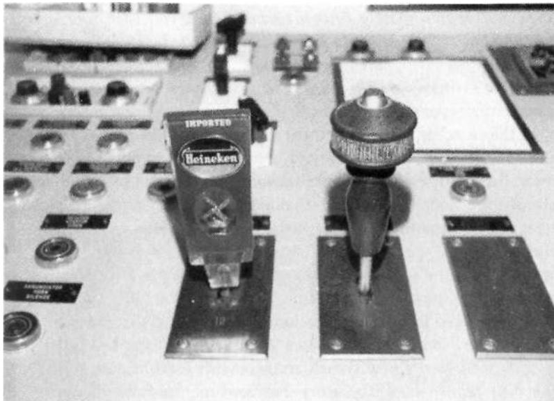
lights being on the ceiling, you have to do a mental rotation of the switches to get them to conform to the lights. The mapping problem is unsolvable with the current structure of switches.
