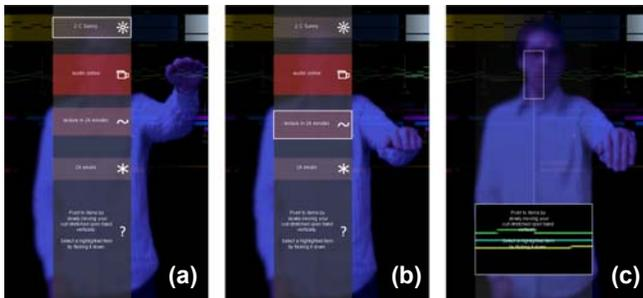
Figure 10. Self revealing help using looping video sequences. In this example, actions with the *palm down* posture is demonstrated during the subtle interaction phase. (a-b) show continuous vertical movement with the *palm down* posture highlighting items. (c) shows the result of selecting the item with a downward flick action.
